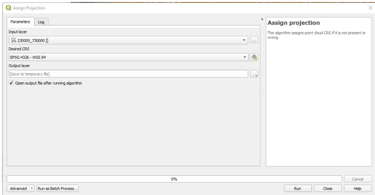
**Figure 4. Assign projection to las algorithm.**
