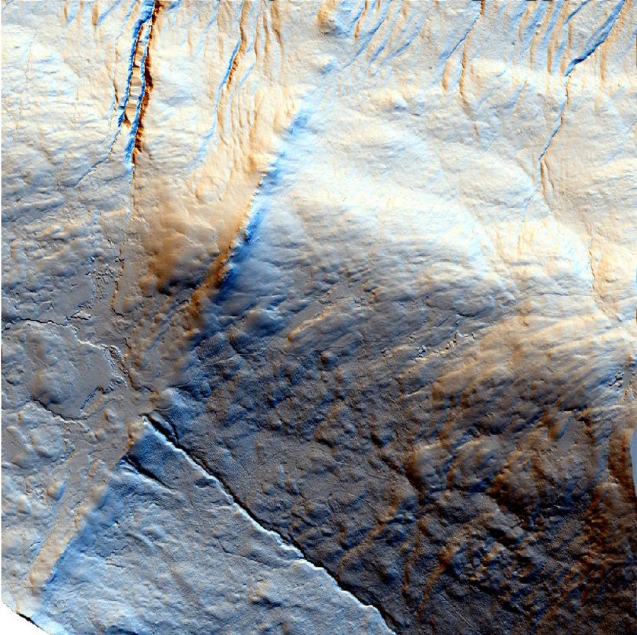
*Figure 12. Multidirectional Hillshade generated from the Relief Visualization Toolbox.*
