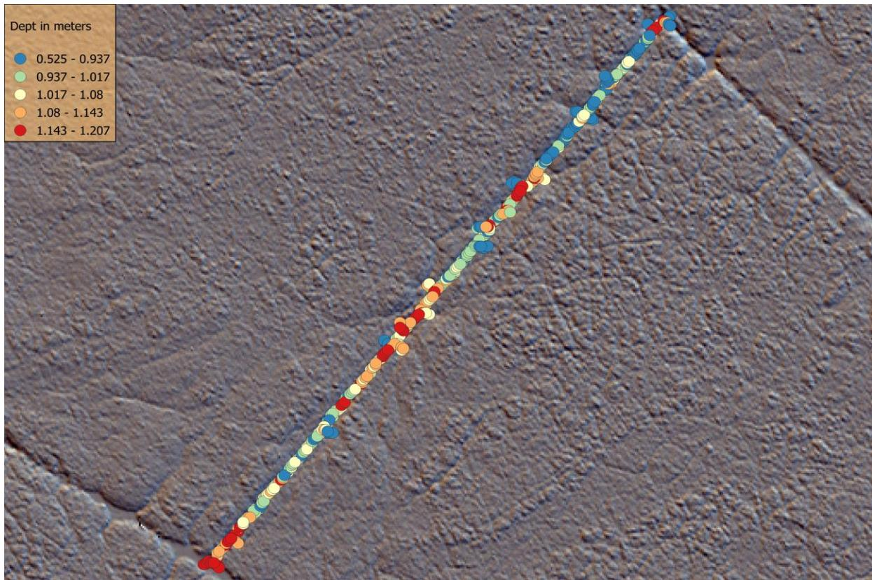
*Figure 30. Calculate depth point of drainage canal.*
