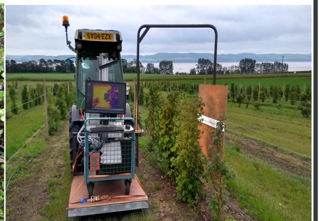
Figure 3. Hyperspectral camera platform being utilised to identify early plant stress signals
