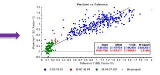
Calibration results for the prediction of Bulk Density (NIR)
