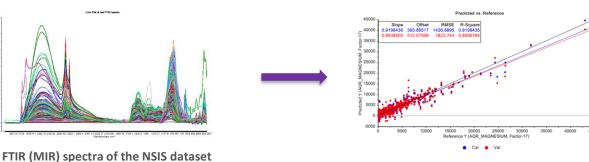
Calibration results for the prediction of Mg (FTIR)
